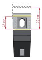
Shelf is clamped between a layer of ridged plastic on the lower side and soft rubber on the upper side (coloured parts).
