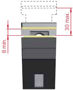
Shelf is clamped between a layer of ridged plastic on the lower side and soft rubber on the upper side (coloured parts).
