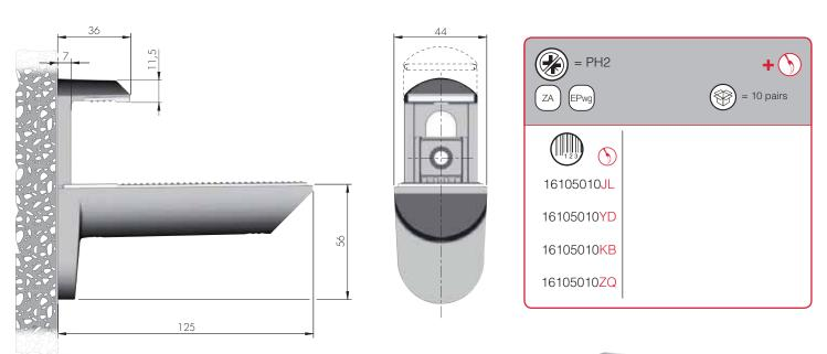
NOTE: KAIMAN MAXI is supplied in carton box including 2 pieces, accessories and fitting guide. Countersunk fixing screws Ø 5x50 and rawlplugs Fischer SX Ø 8x40 to wall are included.
