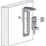
Recommended fixing countersunk screw type - head Ø 5 mm max.
