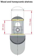
Shelf is clamped between a layer of ridged plastic on both the lower and upper side (coloured parts).
