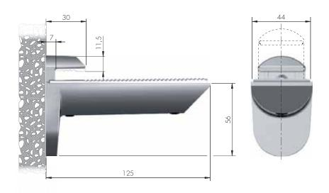
NOTE: KAIMAN is supplied in carton box including 2 pieces, accessories and fitting guide. Countersunk fixing screws  $\varnothing$  5x50 and rawlplugs Fischer SX  $\varnothing$  8x40 to wall are included.
