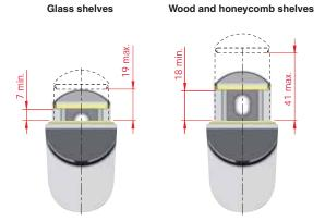
Shelf is clamped between a layer of ridged plastic on both the lower and upper side (coloured parts).
