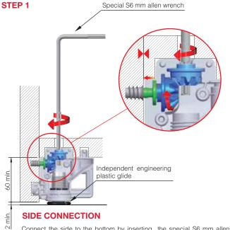
Connect the side to the bottom by inserting the special S6 mm allen wrench with hexagonal bit into the through hole, until it fits into the first cavity.
